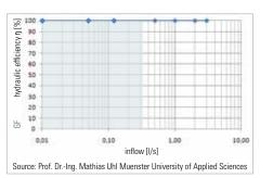
80% of the average intensity of rainfall in Germany is under 15 l/(sxha), resulting a volume flow rate of 0,32 l/s with a roof area of 213 m².
